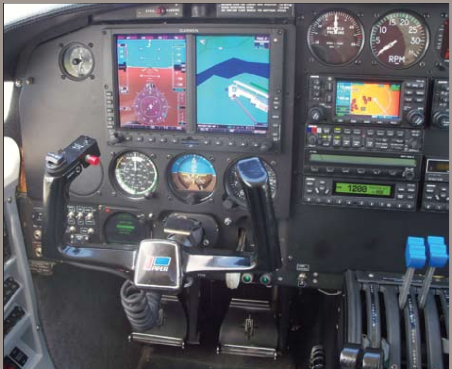
The Piper Navajo panel pictured above didn't look like this when the airplane left the factory. The Garmin G600 replacing steam gauges was added later, at some expense. Buy your step-up airplane with as much of this equipment already installed as you can find.
